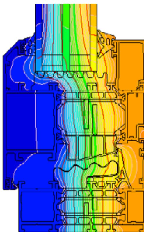
example isotherm arrangement for the frame and window sash assembly of the GN OUTi+ window system (GN521 + GN010)
